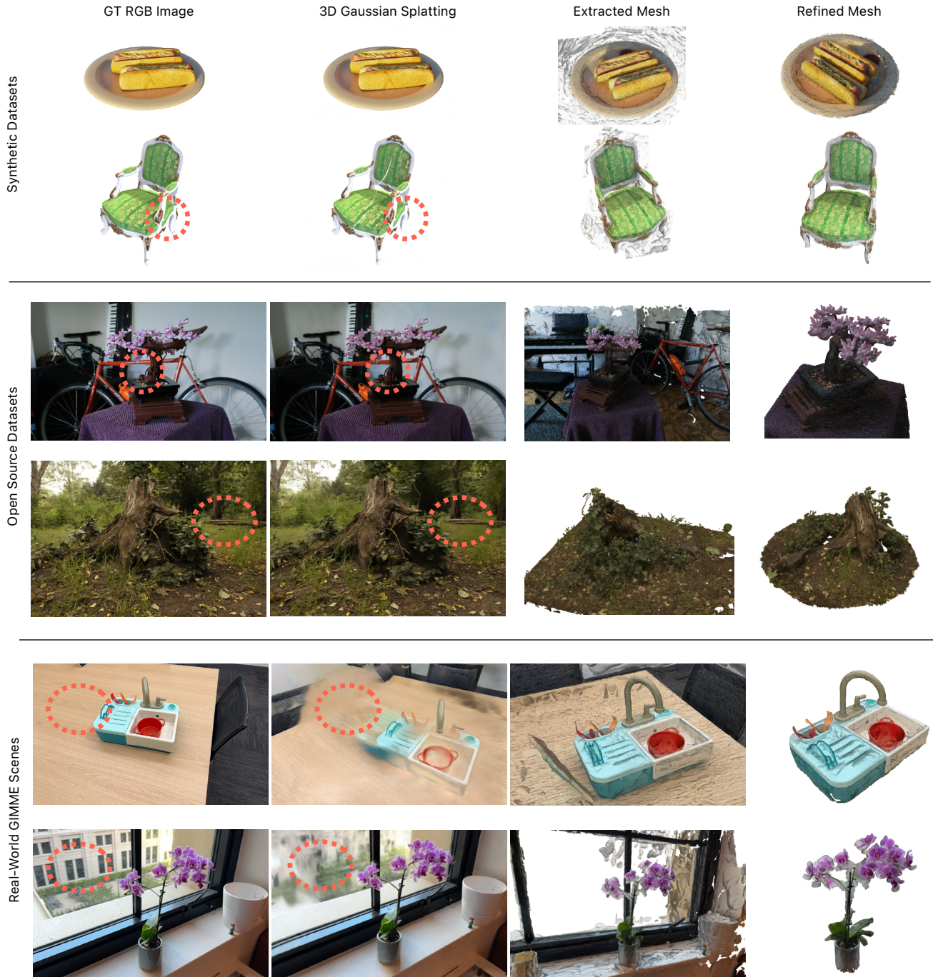
Figure 2. GIMME pipeline. The stages of the GIMME system’s processing pipeline on synthetic, real-world, and self-generated datasets. Note the visual fidelity our system achieves in the final meshes across various datasets. Undesired artifacts, such as discrepancies in texture and geometry, are highlighted with red dashed circles, indicating areas for potential improvement in our pipeline.
